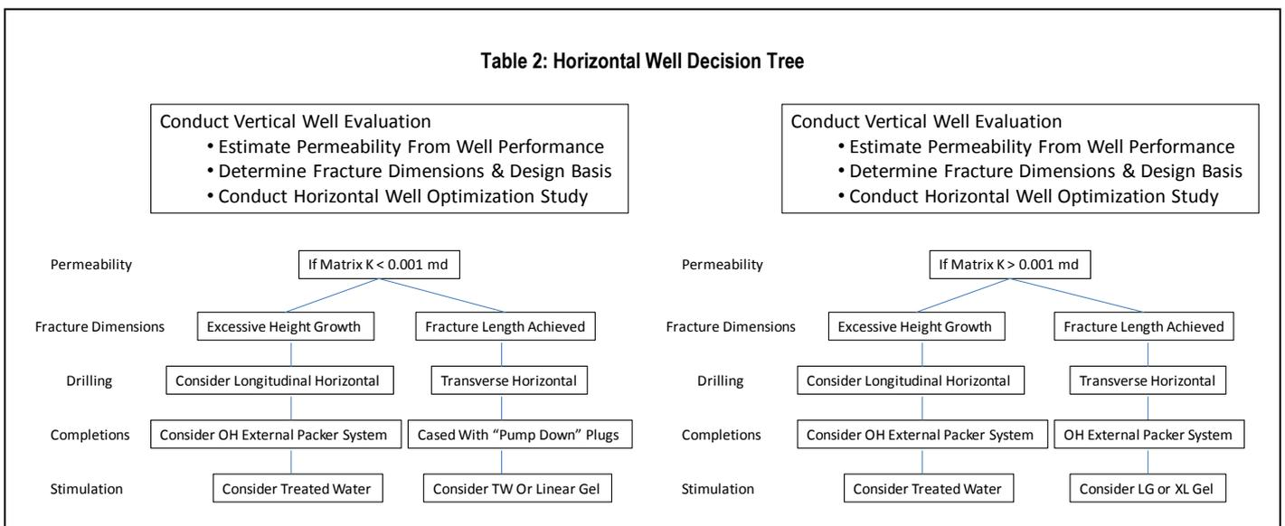
As shown, the data collection plan is based on collecting data in vertical wells. The reason for this is that much of the data we use to evaluate the well is a pressure measurement.
