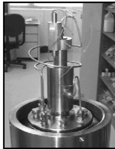
Figure 5: Test Cell Head With Piston and Inlet Ports
